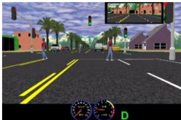
8 - The simulators record reaction times, driving errors and speed exceedances.
