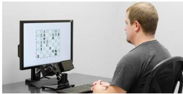
22 - This is a participant sat at the desktop version of an eye tracker. The camera is placed below the monitor and records the pupil diameter and corneal reflection in order to record what they are looking at on the computer screen.
