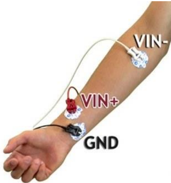
2 - Attachment of electrodes to the forearm.
