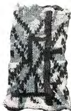
- Domestic Knit Machine - Punchcard design & sublimation Print - Tension 7 - Wool & Polyester
