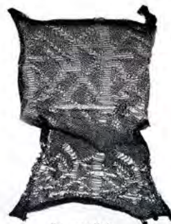
- Domestic Knit Machine - Punchcard Design - Monofilament & Cotton
