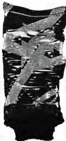
- Domestic chunky knit machine - True rib trim using industrial chunky machine gauge of 2.5 - Punchcard Design & screen printed + foiled my print. - Viscose tape yarn. - Tension 4
