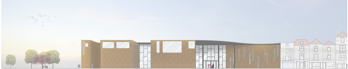
Elevation of the NW façade of the building. Parallel a main road, an oak façade curves to follow the path.
