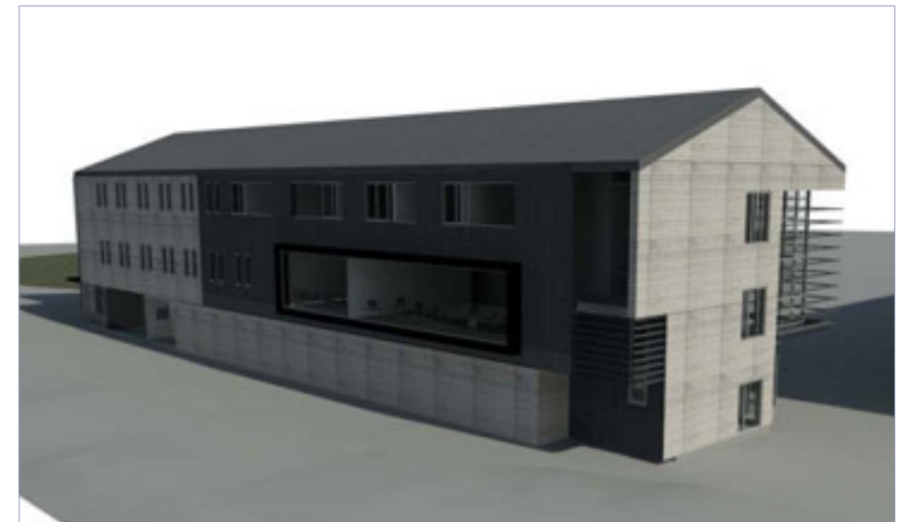
VERSION E - METAL CLADDING WRAPPING DOWN THE NORTH FACADE FROM ROOF TO LEVEL 01. (METAL WOULD BE SET PROUD OF THE TIMBER CLADDING)
