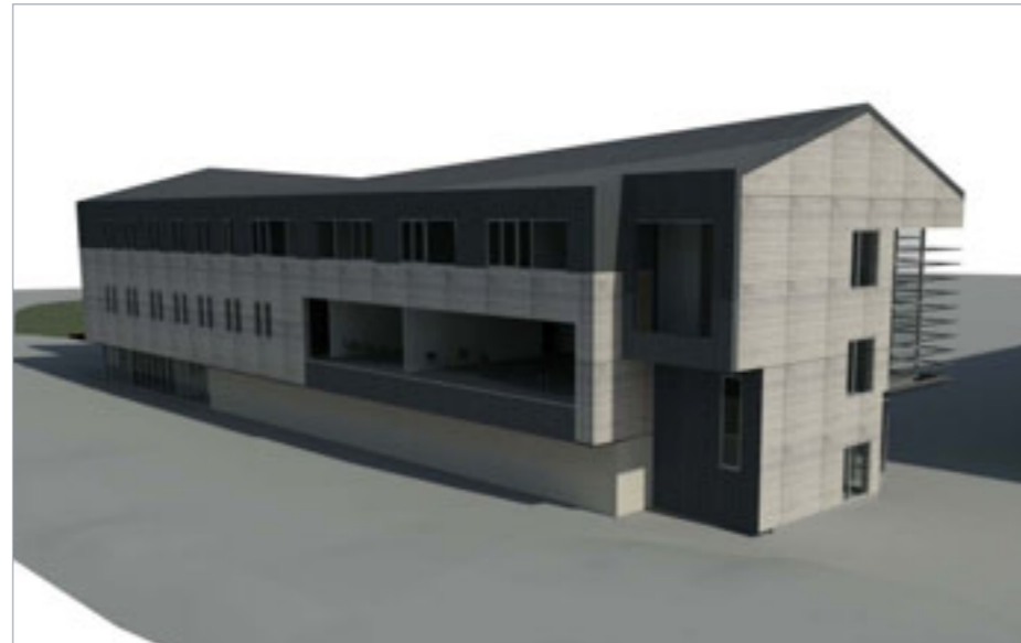
VERSION B - BOWED ROOF PROPOSAL WITH NORTH FACADE ON UPPER FLOORS OFFSET FROM GROUND LEVEL FACADE TO CREATE AN OVERHANG.
