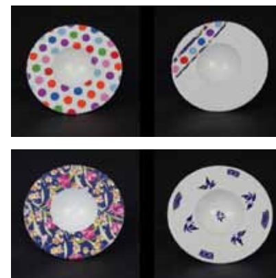
3D printed, fired and glazed ceramic plates, AHRC / CFPR / Denby Project, D. Hudson 2012).
